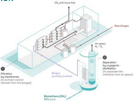
The patented WAGABOX® technology recovers 90% of the methane contained in the landfill gas even with up to 30% air concentration (oxygen and nitrogen). It guarantees the delivery of RNG containing at least 98% methane, which can be injected directly into the local distribution gas network. The 10% remaining methane is used on site to burn any volatile organic compound contained in landfill gas.
